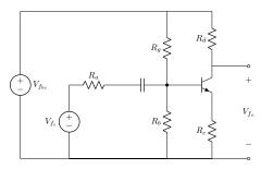
2. In the following circuit, assuming  $\beta \approx \textbf{Beta}$  and that  $V_{be} \approx 0.65V$ , find the value of  $R_g$  such that the DC level of  $V_{f_o}$  is equal to DC level.
